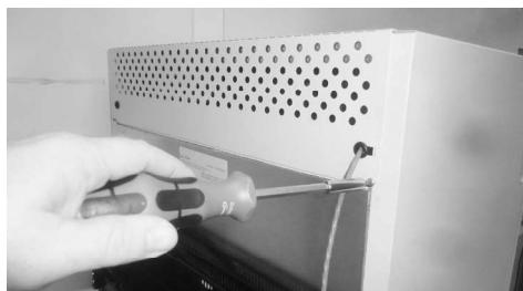
6. Place the top cover in closed position and remount the two screws (TX20).
