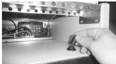
3. Remove the two rubber plugs from the porthole (1 in the top & 1 inside the appliance).
