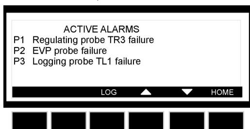
3. Push the **LOG** button to enter the **ACTIVE ALARM LOG**.
