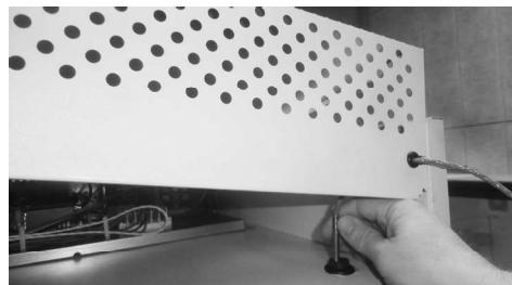
4. Guide the sensor through the top cover protection bushing, through the porthole and into the appliance.
