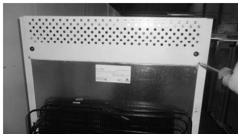
1. Remove the two screws (TX20).
