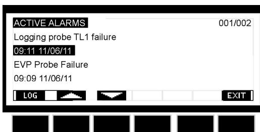
5. Push the **LOG** button to enter the **ALARM LOG**. This menu contains all the memorized alarms. For each alarm the starting time and date and the finish time and date are recorded.
